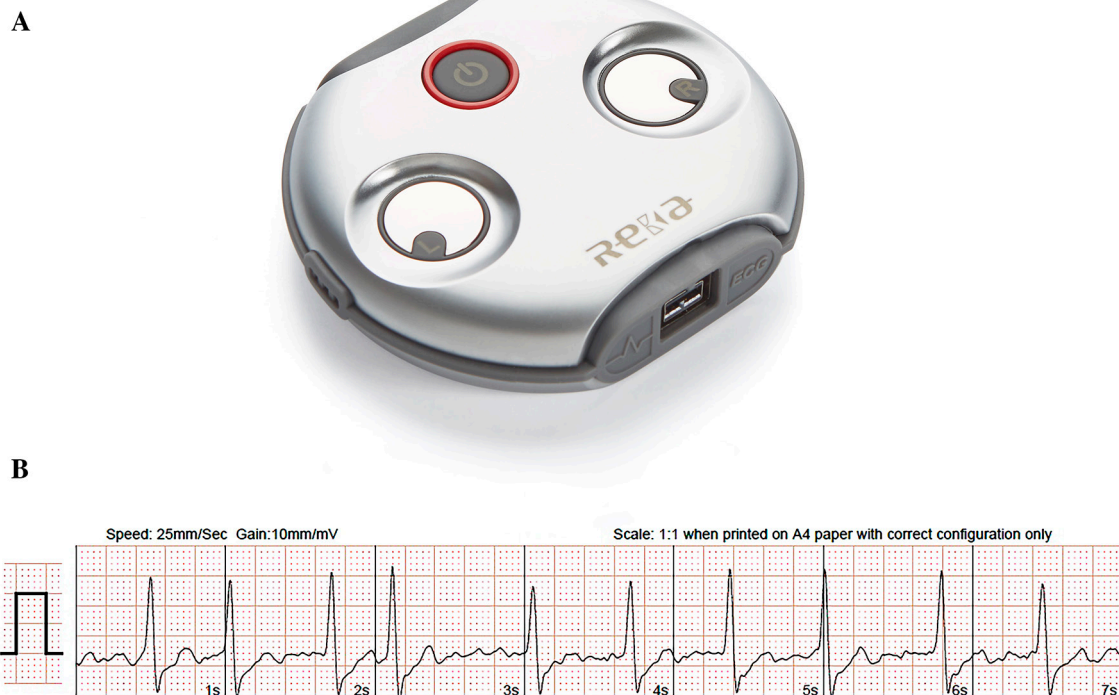
Figure 1 (A) Photograph of the handheld patient-activated ambulatory ECG monitoring device. (B) Example of patient-activated single-lead ECG strip recording during sensation of palpitations.
